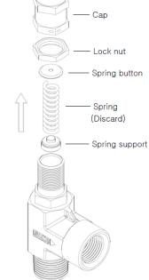
**4.** Insert the spring support, **new spring**, spring button, lock nut and cap into the body.
